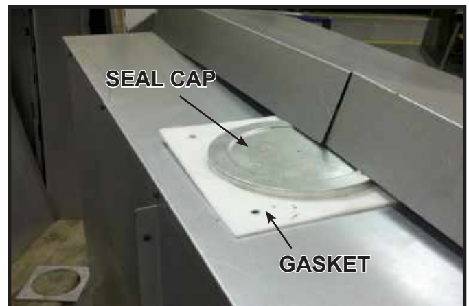
Figure 6.2 Seal Cap and Gasket Location
