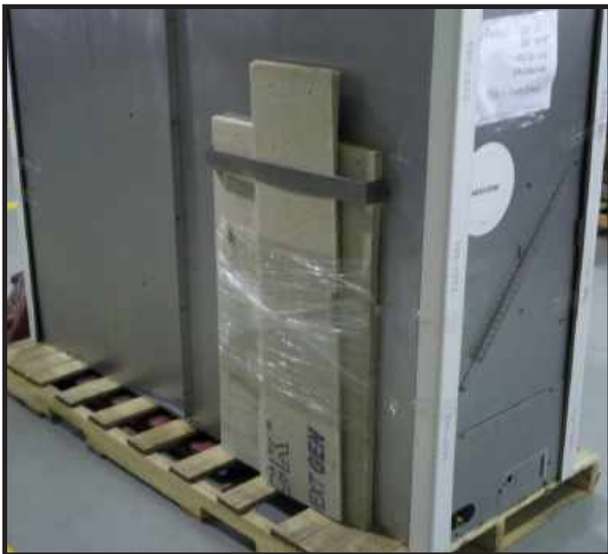
Figure 6.6 Shipping Location of Non-Combustible Board
