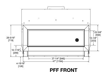
The PFF decorative front has an installed depth of 3/4" [19mm], measured from the front of the non-combustible finishing material to the front of the decorative front.
