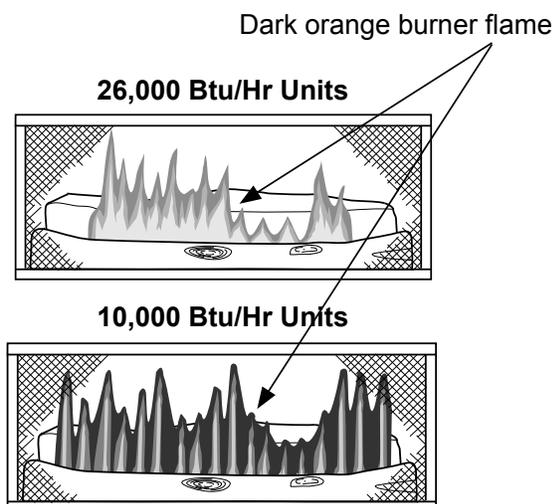
**Figure 41 - Incorrect Burner Flame Pattern**
