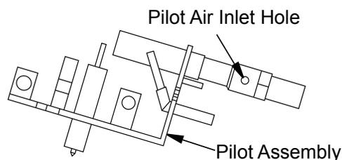
**Figure 43 - Pilot Inlet Air Hole (Propane/LP Gas)**
