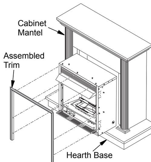
**Figure 13 - Installing Fireplace into Mantel Assembly**
