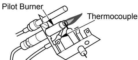
**Figure 38 - Correct Pilot Flame Pattern (Propane/LP Shown)**
