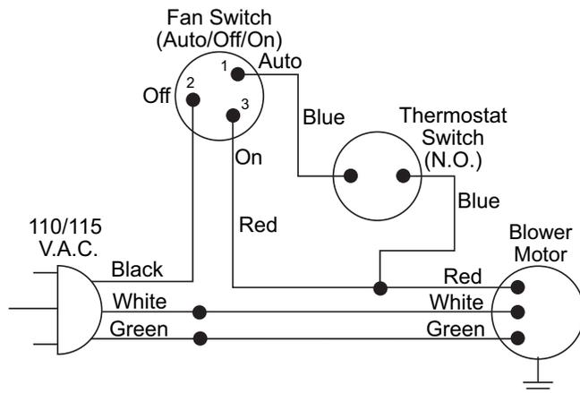
**Figure 17 - Wiring Diagram For Blower Accessory Standard Installation**
