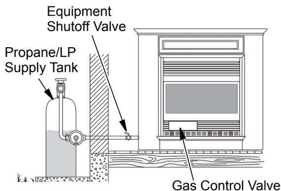
**Figure 26 - Checking Gas Joints (Propane/LP Only)**
