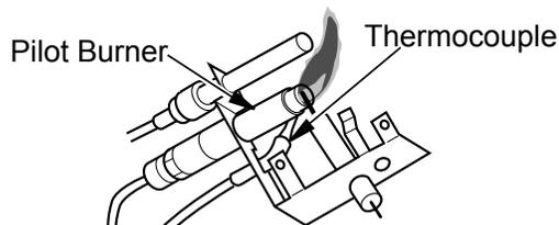
**Figure 39 - Incorrect Pilot Flame Pattern (Propane/LP Shown)**
