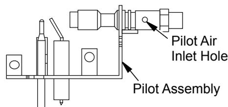
**Figure 44 - Pilot Inlet Air Hole (Natural Gas)**
