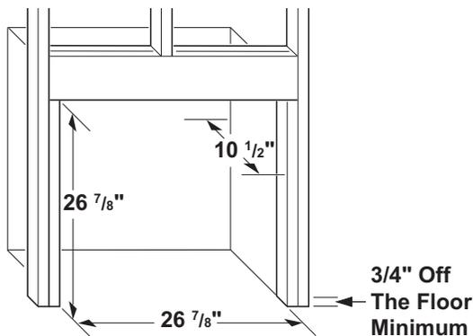
**Figure 7 - Rough Opening for Installing in Wall**
