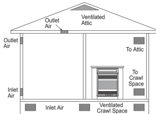
**Figure 5 - Ventilation Air from Outdoors**
