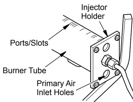
**Figure 42 - Injector Holder On Outlet Burner Tube**
