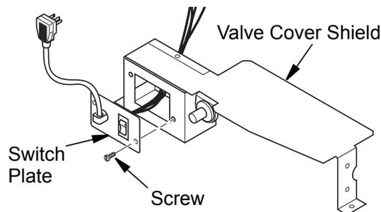
**Figure 18 - Installing Switch Plate to Valve Cover Shield**
