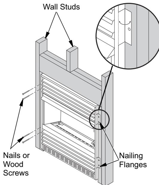
**Figure 9 - Attaching Fireplace to Wall Studs**
