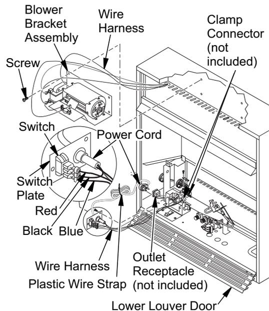
**Figure 20 - Installing Blower Bracket Assembly**
