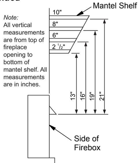
**Figure 10 - Minimum Mantel Clearances for Built-In Installation**
