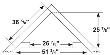
**Figure 8 - Rough Opening for Installing in Corner**
