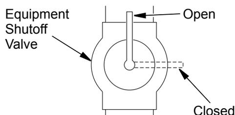
**Figure 25 - Equipment Shutoff Valve**
