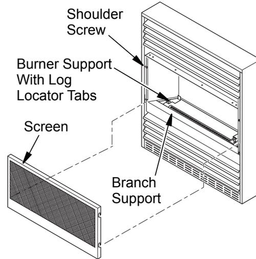
**Figure 2 - Removing Screen**
