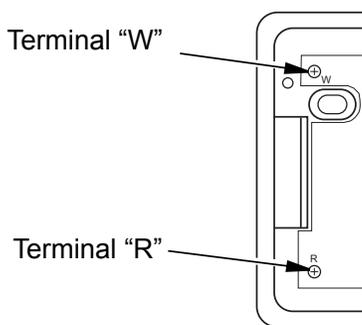
**Figure 31 - Thermostat Base Terminals "W" and "R"**
