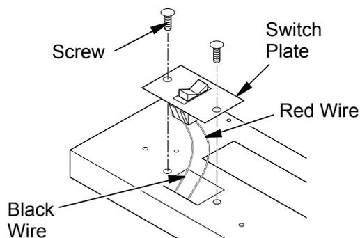
**Figure 28 - Switch Plate and Wiring Harness**
