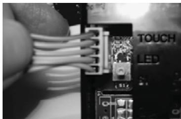
**Figure 27 - Connecting end of Touch Pad Cable**
