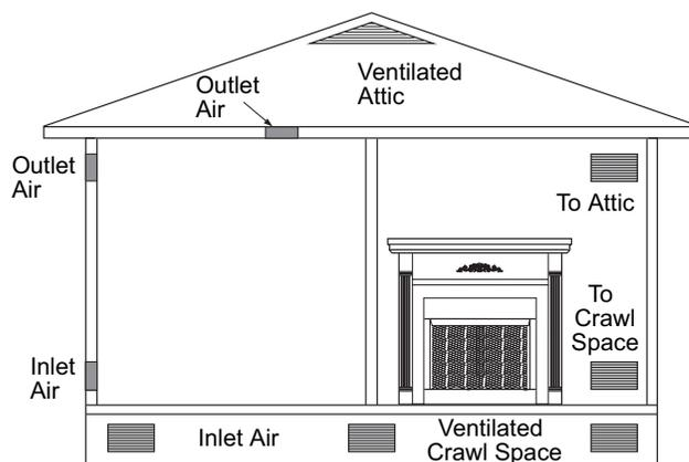
**Figure 5 - Ventilation Air from Outdoors**
