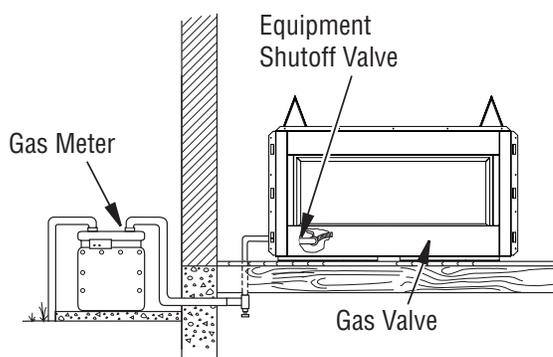
**Figure 13 - Checking Gas Joints for Natural Gas Fireplace**
