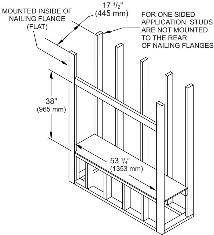
**Figure 2 - Framing Clearances for One Sided Application**
