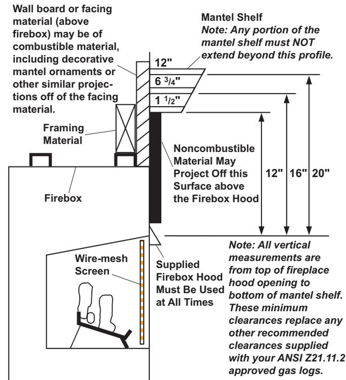
**Figure 7 - Minimum Mantel Clearances for Built-In Installation**
