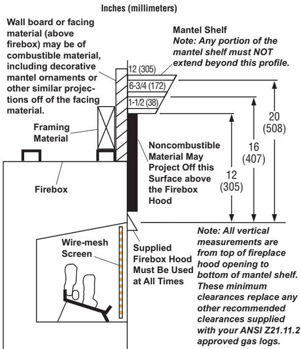
**Minimum Wall and Ceiling Clearances (see figure below)**
