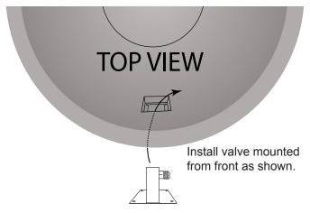
Fig. 7 Top view of MT mounting plate into bowl.
