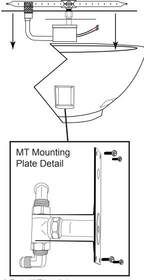
Fig. 6 Typical MT installation.
