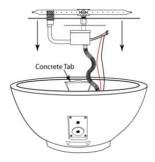
Fig. 10 Installing burner assembly into the bowl.
