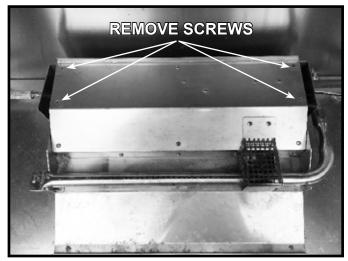
Figure 1. Remove Screws
