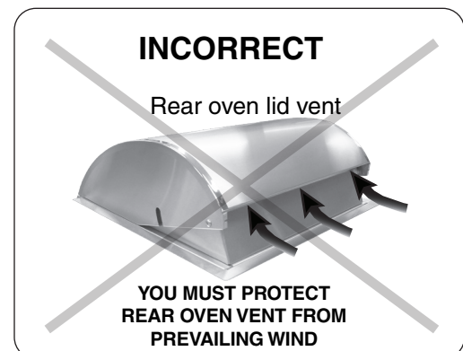
Fig. 10-4 Airflow direction - INCORRECT
