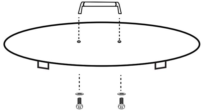
**Fig. 1** Installing handle, screws, washers on lid.
