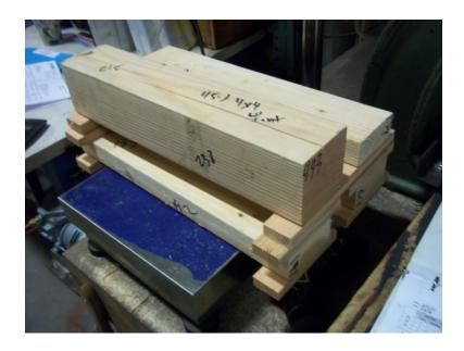
Fuel consisted of 2"x4"x17.5" and 4"x4"x17.5" Green, Douglas fir. Detailed fuel load specifications for each run can be found in the corresponding digital folders submitted with this report.
