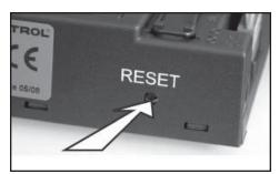
Fig. 2-1 Receiver reset button
