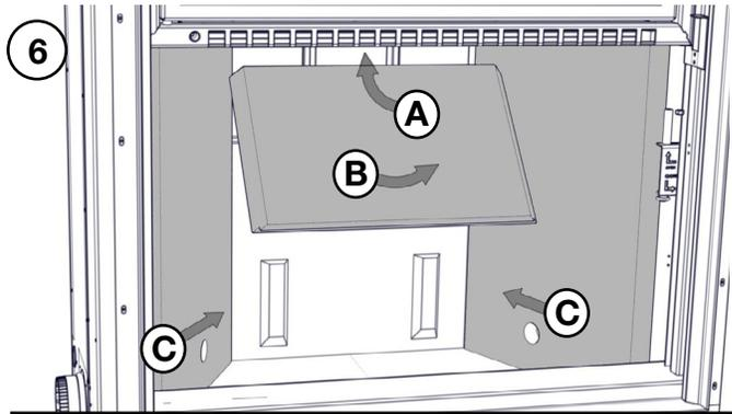
Place and slide the top rear firebrick against the wall (A and B). Push side bricks back to help hold rear bricks in place (C).
