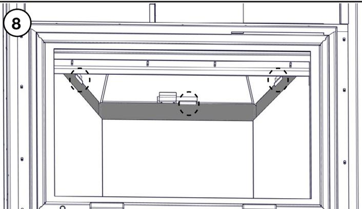
Install the 3 fiber panels and secure with retaining brackets.
