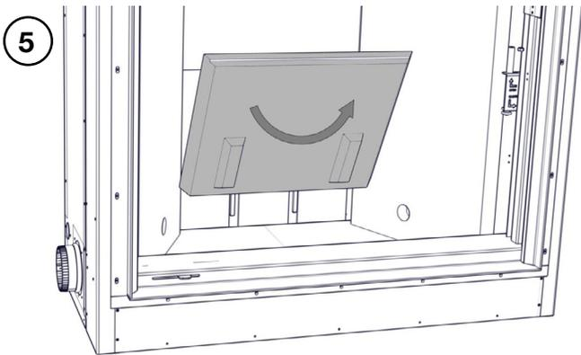
Place and slide the bottom rear firebrick against the wall.
