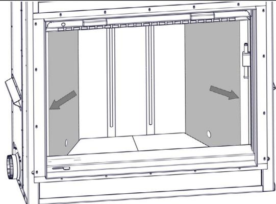
Tilt and install the right and left side firebricks against the wall. To install rear bricks, the side bricks must be pulled forward.
