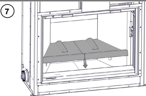
Install the bottom firebricks to lock all firebricks in place.
