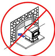
**This stove is not approved to be installed inside a masonry fireplace.**
