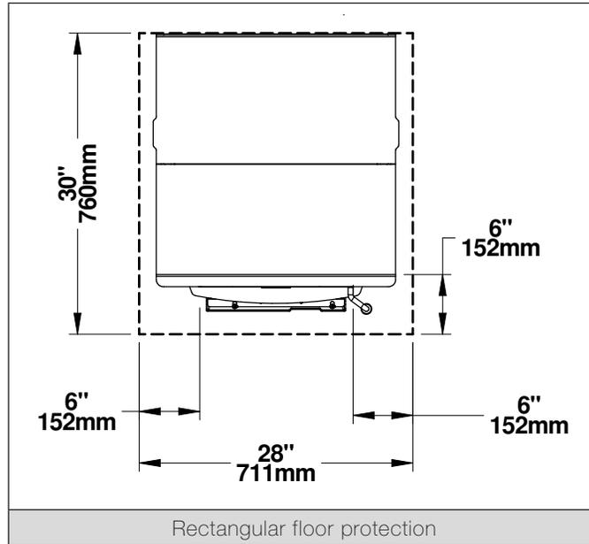
Floor protection must extend at least 6" (152 mm) in front of the loading door opening and 6" (152 mm) on each side of the loading door. It must also extend at least 2" beyond each side of any horizontal venting pipe.
