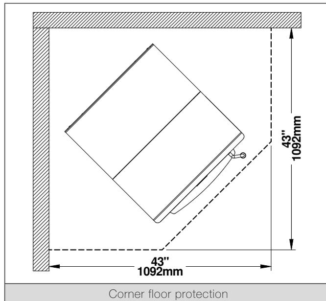
*Note: In Canada, the dimensions of the floor protection shown in the previous image can be used ONLY if opening the appliance door or removing the ash drawer is done when the appliance is OFF completely, meaning there is no more fire in the combustion pot and the blowers are off. In all other cases, see CSA B365.*
