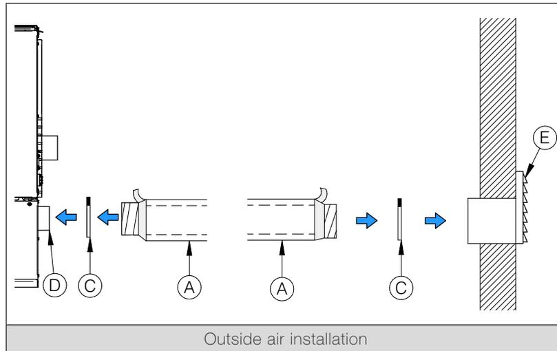
3. From outside, place the outside air register **(E)** in the hole (open side down) and fasten the register to the wall, with screw.
