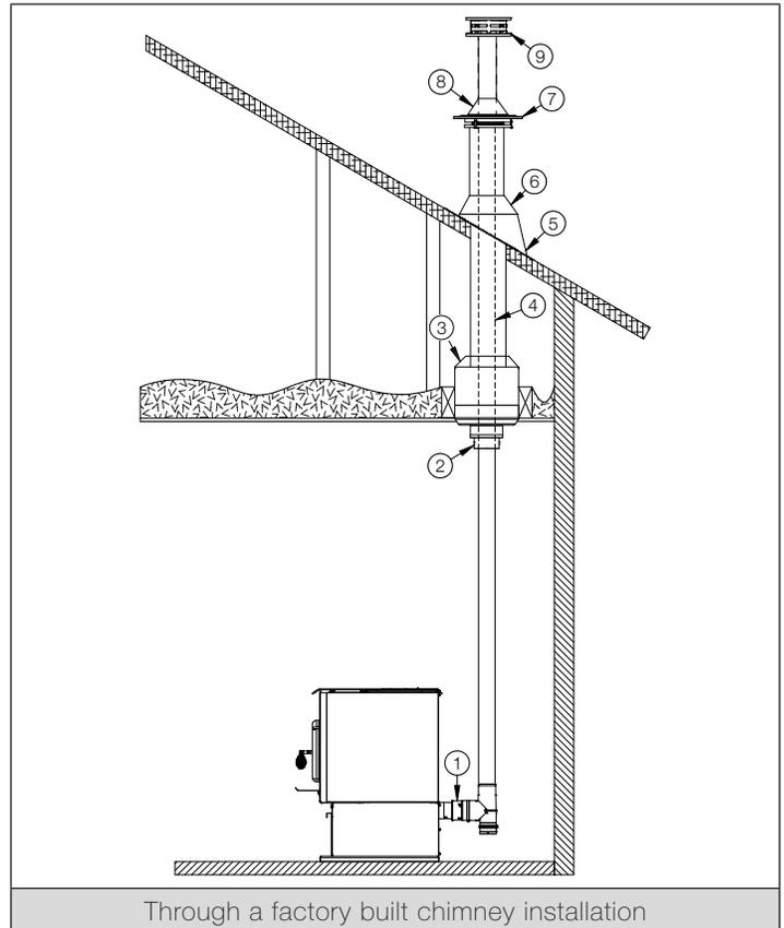
1. Remove any existing chimney pipe from the heater to the universal adapter already installed in the ceiling support.
