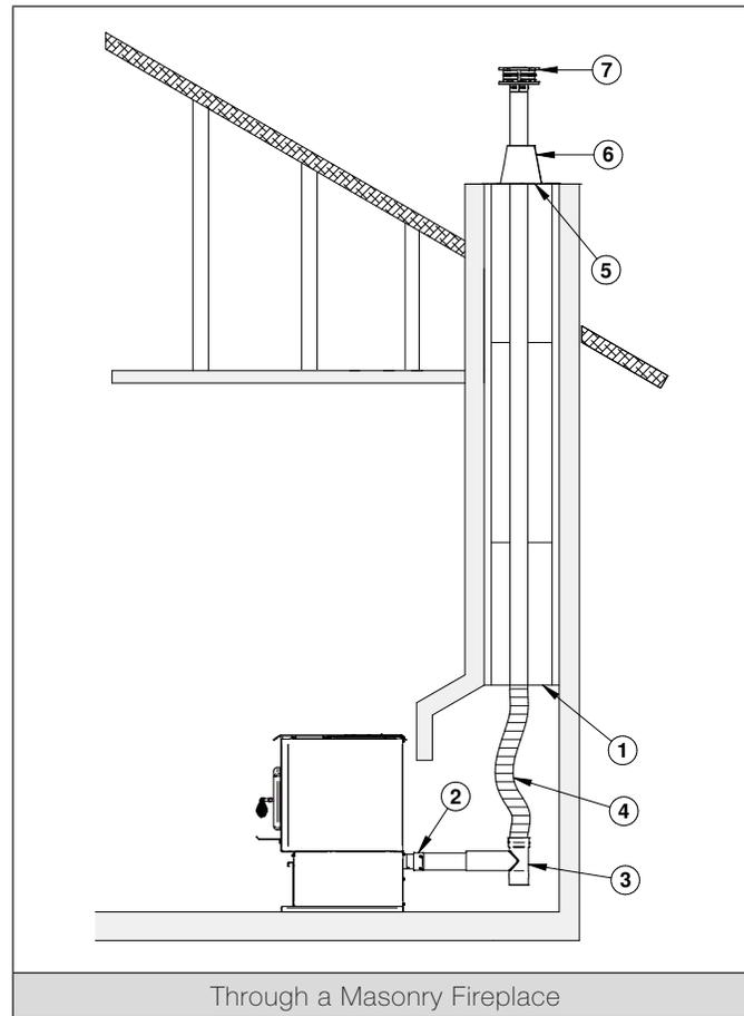
1. Build and install a blocking plate **(1)** inside the chimney to seal the fireplace damper. Stainless steel plate and screws are recommended. Cut a hole for the exhaust pipe. If needed, cut a second hole for the air intake pipe.
