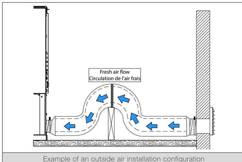
1. Install a 3" inside diameter, either flexible or rigid, insulated pipe (HVAC type, must comply to ULC S110 and/or UL 181, Class 0 or Class 1) to the fresh air intake. **(D)**. To do so, carefully pull back the insulation and plastic cover, exposing the flexible pipe. Attach the flexible pipe using pipe clamps **(C)** or foil tape.
