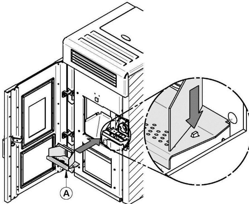
3. If necessary, clean the air intake channel. To reach the air intake channel clean out trap, open the door and remove the ash drawer.
