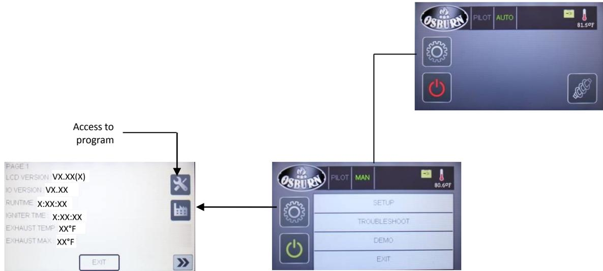
Page 1 provides information on the software version of the stove's two electronic cards. In addition, you have the total number of hours your stove has been in operation, the temperature of the exhaust gases and the maximum temperature that your stove has reached.
