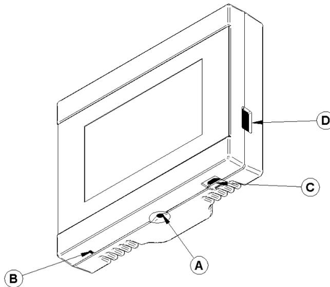
3. Press on the button (A) at the bottom of the screen to turn off the screen.
