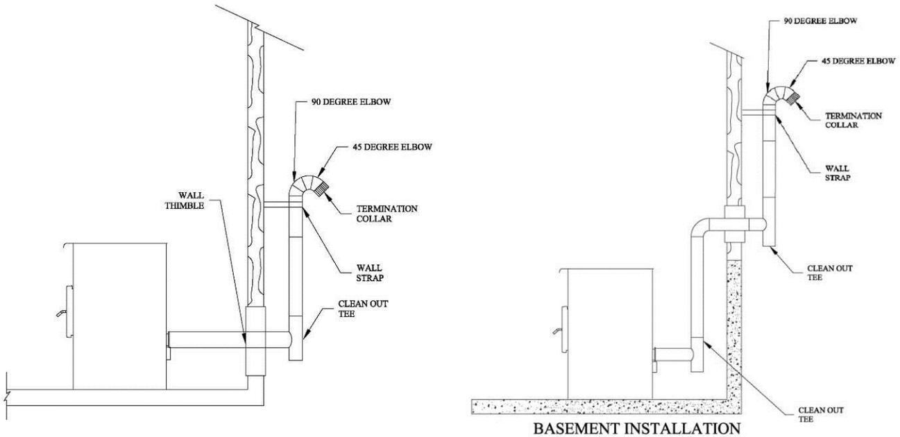
1. Position stove following clearances given in **Section 3: Clearances to Combustible Material** and following vent manufacturer's instructions. Then locate the position of the exhaust pipe in the wall.
