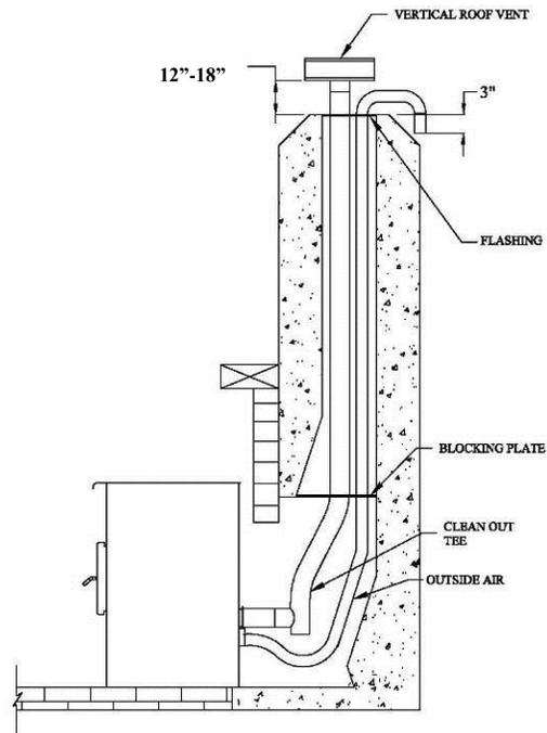
**NOTE: THE STRUCTURAL CONDITION OF THE MASONRY CHIMNEY MUST FIRST BE INSPECTED BY A QUALIFIED CHIMNEY SWEEP OR INSTALLER.**
