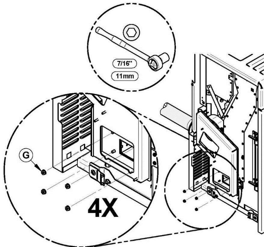
Remove the duct assembly
