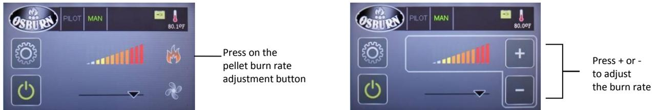
The stove's input range goes from 10,000 BTU/h to 45,000 BTU/h. To change combustion level, select the flame icon
