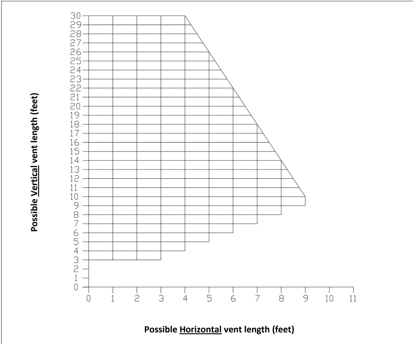
For example, let's imagine an installation consisting of a horizontal vent coming out at the back of the stove on a total distance of 8 feet. This horizontal run is followed by a tee and a 6-foot vertical rise. This type of installation is not acceptable. As you can see, the vent termination is clearly outside the allowed configuration zone on the chart because the venting system proposed **does not have at least one foot of vertical rise for each foot of horizontal run.**
