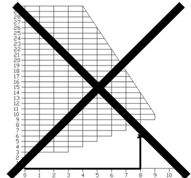
Instead, if the installation consisted of a horizontal vent coming out at the back of the stove on a total distance of 4 feet, followed by a tee and a 6-foot vertical rise, it would be acceptable. The installation end should be within the allowable configuration zone on the chart since it would have at least one foot of vertical rise for each foot of horizontal run. Furthermore, the total vertical rise would be at least 3-foot high.
