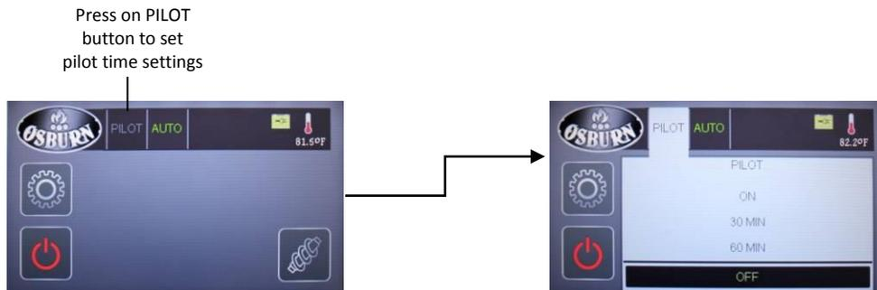
**Note:** Pilot feed rate is lower than the minimum combustion level feed rate.
