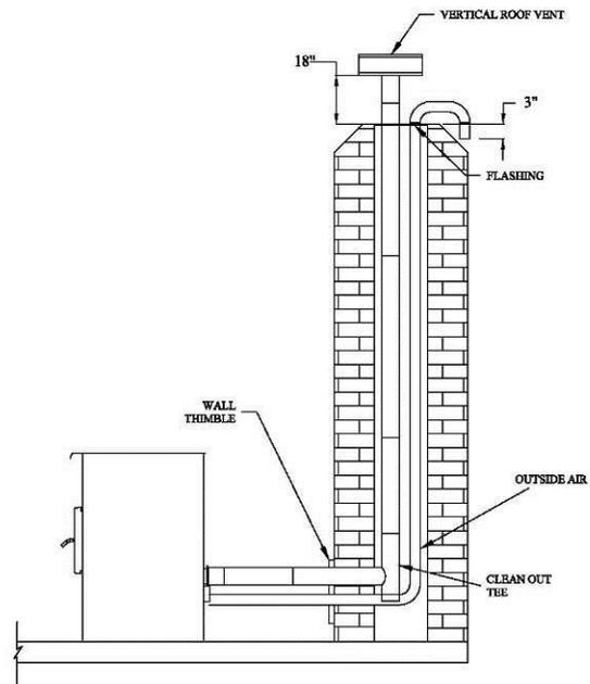
5. Install the cleanout tee at the bottom of the vertical vent system and lower it down the chimney until the center branch of the tee is aligned with the hole in the masonry.
