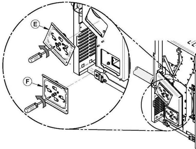
Locate both openings. Using the provided scraper, remove the dirt in the bottom channel of the heat exchangers. Use an ash vacuum to complete the cleaning operation.
