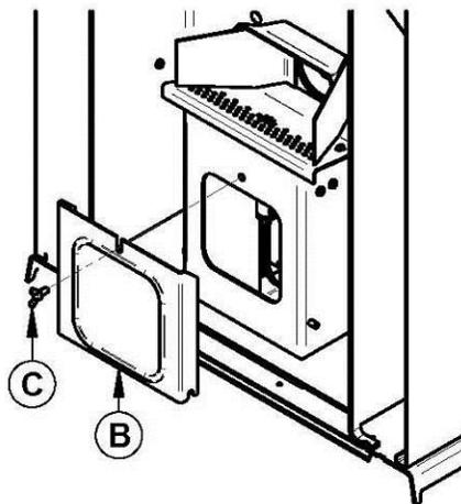
5. Verify that the clean out trap gasket is still in good condition; replace it if needed (3/16" black round gasket (AC06815)).
