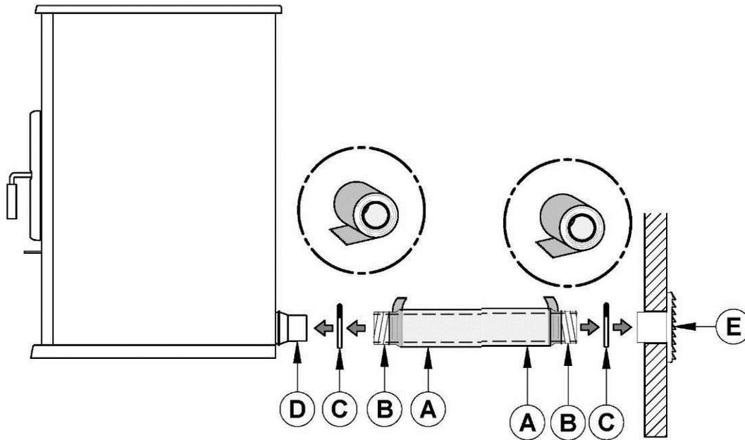
A rodent guard (minimum 1/4" wire mesh) must be used at the termination. All connections must be secured and airtight by either using the appropriately sized hose clamp and/or UL-181-AP foil tape.
