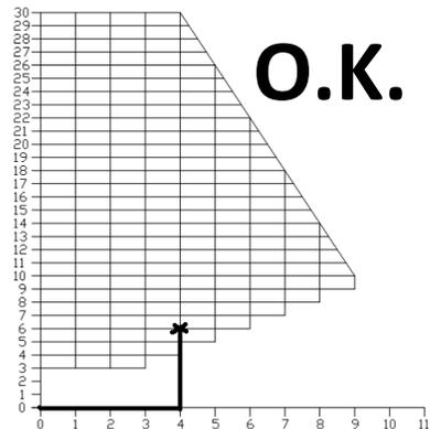
**WARNING:** To reduce the risk of smoke spillage there should always be at least one foot of vertical rise for each foot of horizontal run. In all cases, at least 3 feet of vertical rise is needed.
