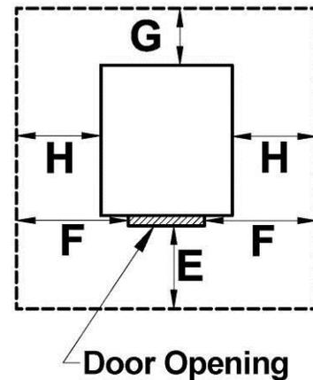
**CAUTION: THE STOVE MUST BE PLACED ON A CONTINUOUS (GROUTED JOINTS) NONCOMBUSTIBLE MATERIAL SUCH AS CERAMIC TILE\*, CEMENT BOARD, BRICK, MILLBOARD OR EQUIVALENT, OR ANY OTHER APPROVED OR LISTED MATERIAL SUITED FOR FLOOR PROTECTION.**
