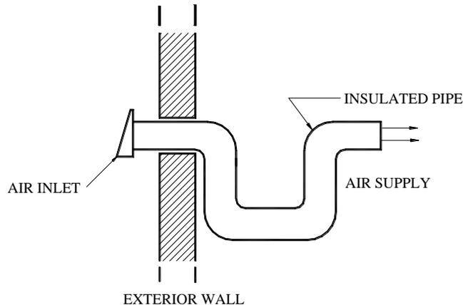
A 3" inner diameter metallic insulated pipe **(A)**, flexible or rigid, must be connected to the fresh air intake adapter **(D)** (this pipe must be HVAC type pipe and must comply with ULC S110 and/or UL 181, Class 0 or Class 1 Standards and must withstand temperatures up to 250 °F).
