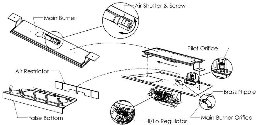
1. Remove [3]screws from false bottom. Remove the false bottom and air restrictor.
