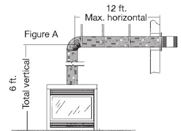
**NOTE:** The final location of the fireplace must be such that the horizontal vent dimensions fall within those stated on the graph. The Maximum Vertical vent run is 40ft. (12.2 meters).
