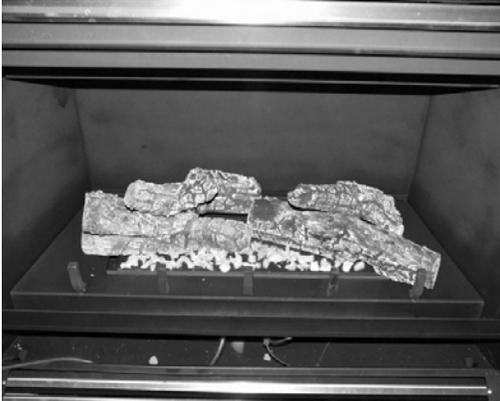
**STEP 8** - Break glowing ember insulation into 1/4" pieces. Place embers onto front burner but ensure you do not cover air slot that is located between front burner and false bottom.
