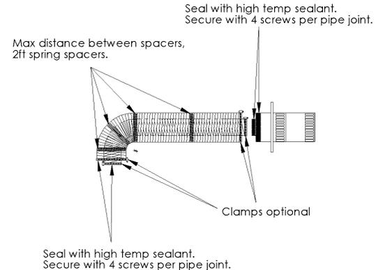
**NOTE:** It is critical to the proper and safe operation of this fireplace that on all connections the inner liner and the outer casing are both caulked with liberal amounts of sealant. Do not use any kind of tape or silicone other than that recommended in this manual, Mill Pac Sealant
