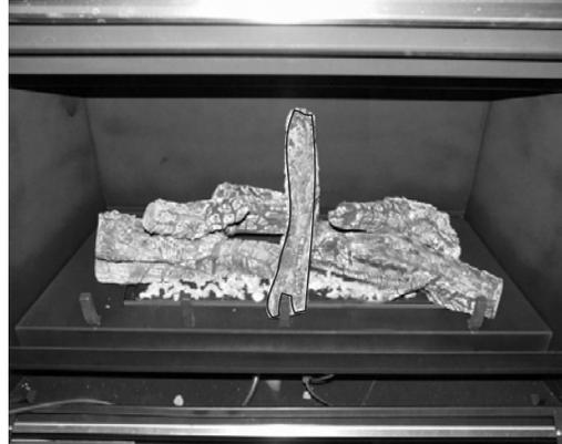
**STEP 9** - On Log #5, you will find a location slot that will align with the middle grate bar. Slide into place and rest Log #5 onto Log #2's flat area.
