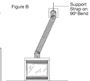
It is recommended for **Propane Horizontal Installations** that the venting should be a minimum of one foot vertical off the flue before the elbow on any horizontal runs of one foot or greater. This allows for cleaner combustion and greatly reduces carboning and cleaning of glass. (Does not apply to Back Flue Models).
