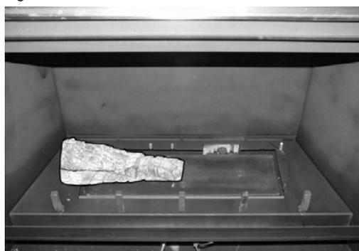
**STEP 4** - Locate left side Log #1 locator tab. Place Log #1 onto locator tab by aligning placement hole on the underside of Log #1 with tab.
