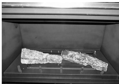
**STEP 5** - Locate right side Log #2 locator tab. Place Log #2 onto locator tab by aligning placement hole on the underside of Log #2 with tab.
