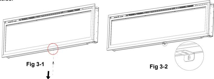
**B**.Using the screw previously removed, attached the L-bracket (supplied) to the bottom of the fireplace box.(**Fig 3-2**)
