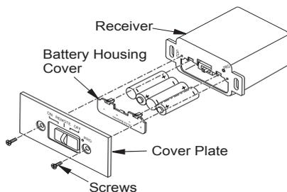
**Figure 22 - Battery Install Remote Control Receiver**
