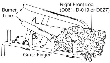
*Figure 24 - Installing Right Front Log*
