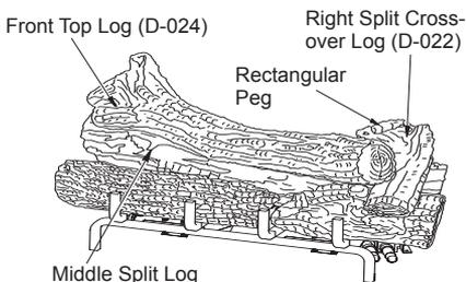
**Figure 30 - Installing Large Middle Log**
