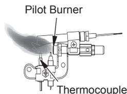
Figure 50 - Incorrect Pilot Flame Pattern
