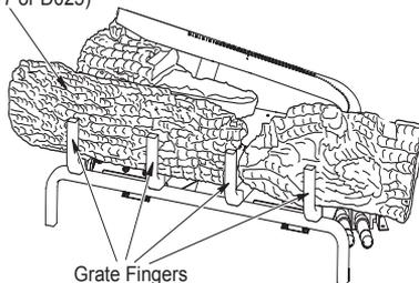
**Figure 26 - Installing Front Left Log**
