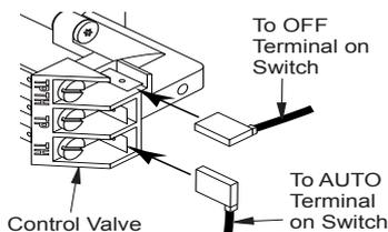
**Figure 18 - Connecting Wires**
