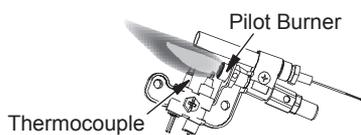
Figure 49 - Correct Pilot Flame Pattern
