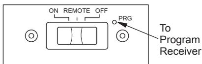
Figure 48 - Programming Remote Control to Receiver
