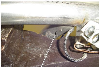
Vertical Portion of Burner Tube
